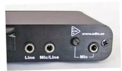
Plug the other end of the patch cord into the "Line" or "Mic/Line" jack on the back of the Univox DLS-50. (They are the same internally although they are labeled differently, so it doesn't matter which one you use.) Note: Don't connect **audio/line outs** to the "Mic" jack, only mic outs, or you risk blowing your Univox DLS-50.
