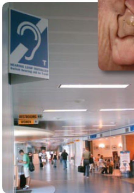
HEARING AIDS with an embedded "T" switch (for telecoil) can pick up clearer sound in the Gerald R. Ford International Airport in Grand Rapids, Mich., which has an induction-loop system (identified by blue signs).
